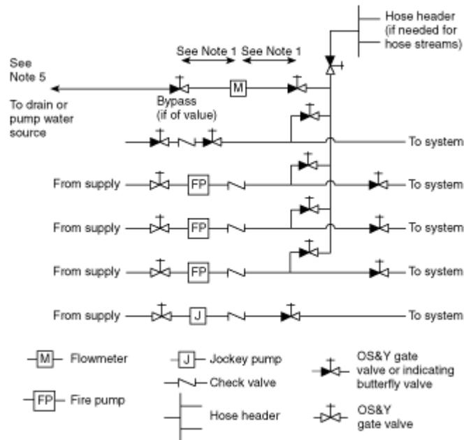
**Figure A-2-14.1.2(b) Typical arrangement for measuring fire pump water flow with meter. Discharge from the flowmeter is recirculated to the fire pump suction line.**
