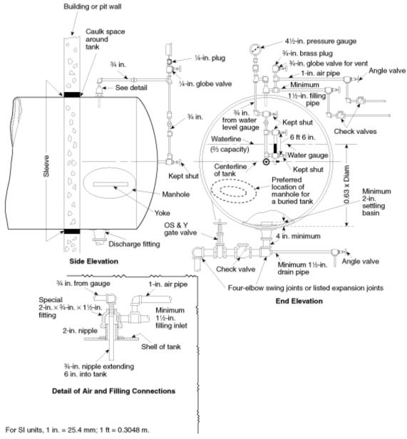
Figure B-2 Alternate connections for pressure tanks.
