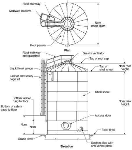
Figure B-14(c) Flange-jointed bolted steel tank.
