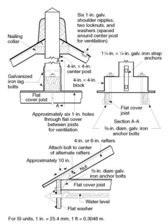
Figure B-4 Section of conical roof.
