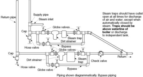
should be installed at same level as main return piping from steam supply pipe and radiator heater.
