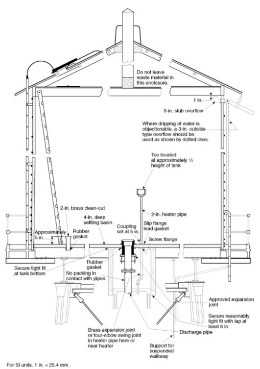
Figure B-12 Typical tower-supported double-ellipsoidal tank.
