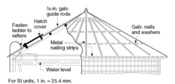
Figure B-5 Typical installation details of an embankment-supported coated fabric suction tank, including fittings.
