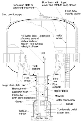
Figure B-13 Typical pedestal tank.
